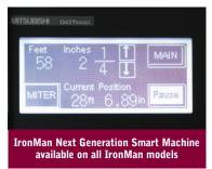
Use the touch screen to automatically control product length, add for miters, if applicable, and keep a total of daily material ran and total footage. Password protected.
